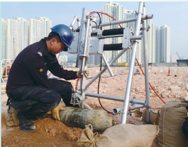
爆炸品处理课人员利用水力磨沙切割系统处理一枚美军 100 磅空投炸弹。 An Explosive Ordnance Disposal officer renders a 100-pound aircraft bomb safe with the assistance of the Abrasive Water Cutting System.
