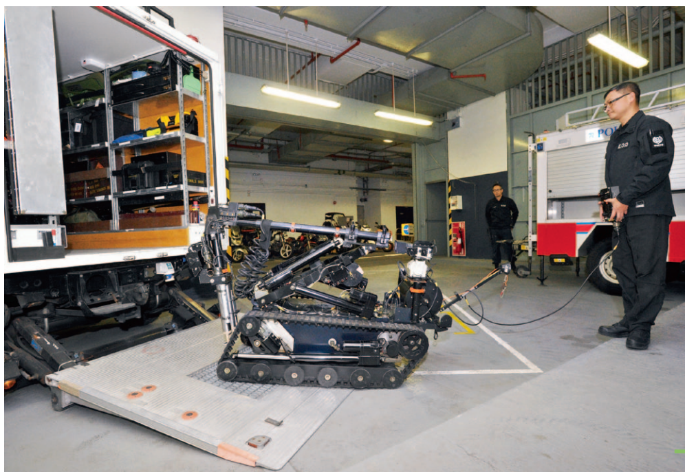
爆炸品处理课人员操作土制炸弹处理机械人「威霸龙」。 An Explosive Ordnance Disposal Bureau officer demonstrates the Improvised Explosive Device Disposal Robot WHEELBARROW.
