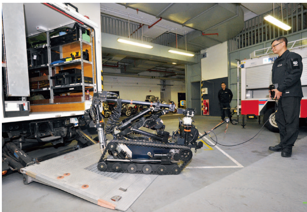
爆炸品處理課人員操作土製炸彈處理機械人「威霸龍」。 An Explosive Ordnance Disposal Bureau officer demonstrates the Improvised Explosive Device Disposal Robot WHEELBARROW.
