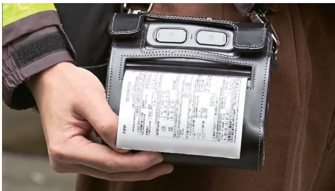
警務人員使用便攜式打印機列印電子告票。 An officer prints out an e-Ticket with a portable printer.
